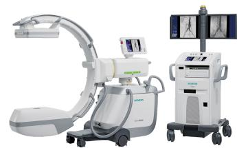
A C-arm comprises a generator (X-ray source) and an image intensifier or flat-panel detector. The C-shaped connecting element allows movement horizontally, vertically and around the swivel axes, so that X-ray images of the patient can be produced from almost any angle.
